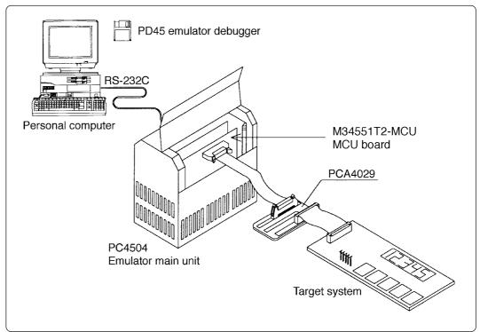
Figure 4.1 Development support system configuration
